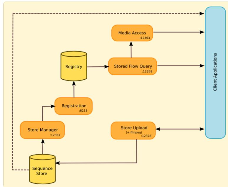
Figure 6: Diagram of the initial implementation of a Media Access API in IP Studio, which can handle import/export of files and reception/transmission of Flows.
