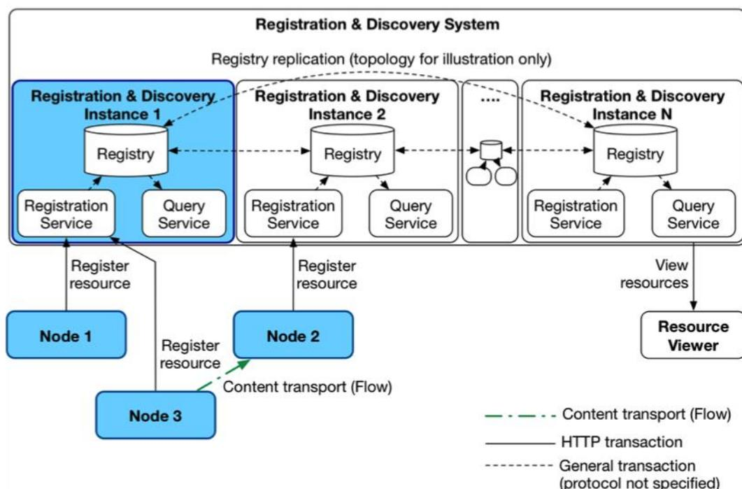
Figure 3: Diagram of three registration and discovery instances configured using the registered model. Nodes can register themselves using any of the instances, and are then visible to all other nodes. Content is transported directly between Nodes.
